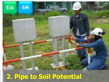
2. Pipe to Soil Potential
